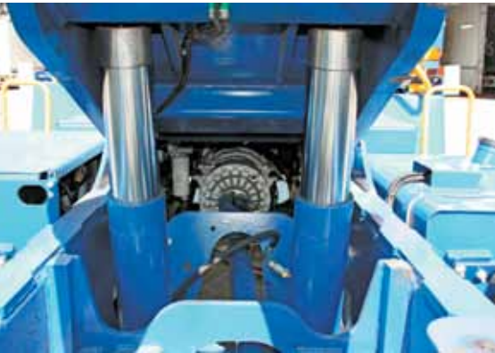
Twin 120mm lift rams help keep things stable under load
