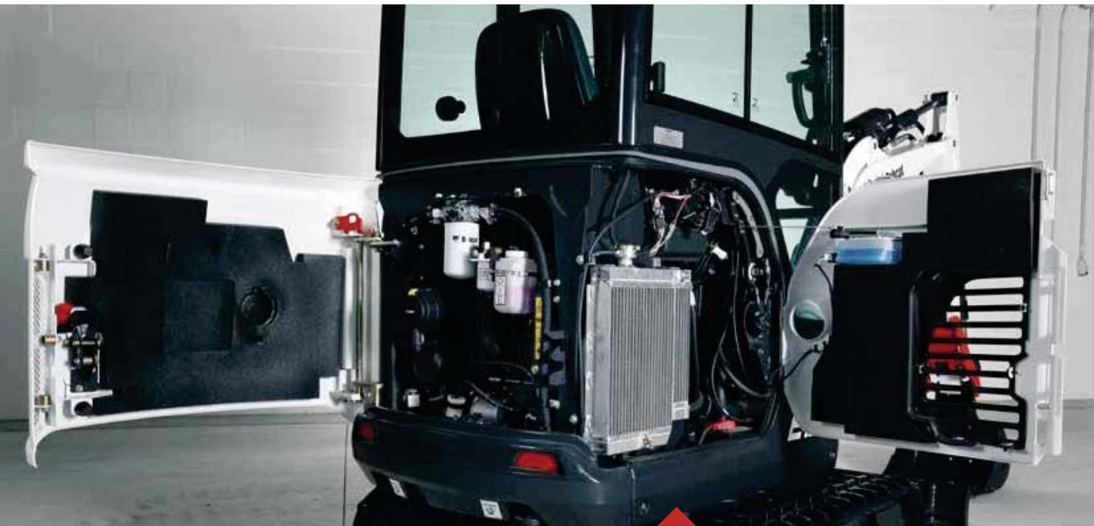
Side-by-side coolers for easy cleaning. Diagnostics are easy thanks to display error codes on control panel and service tool connection. The E20 tailgate provides great access to all daily maintenance components and service points.
