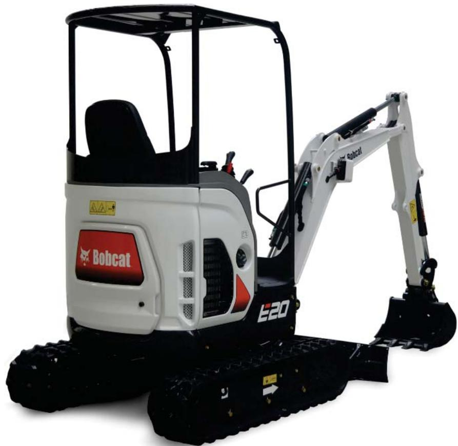
The Zero House Swing (ZHS) concept enhances Zero Tail Swing (ZTS) functionality by further protecting the front upper structure corners turning within the swing circle. ZHS functionality provides 320° of free rotation while working close to any object.
