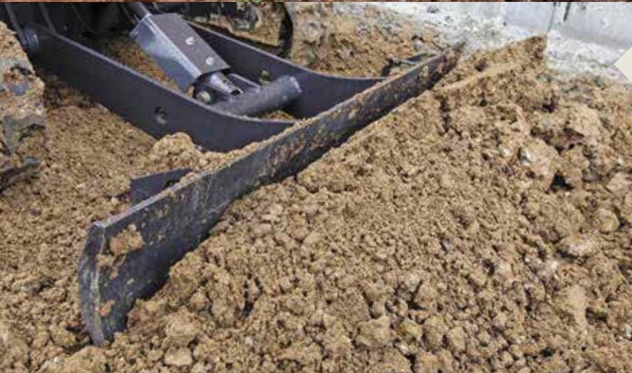
Dozer blade length designed for customers that prefer compactness for working in reduced spaces.
